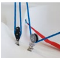
Possibility to put in a ratchet block to create a regatta mainsheet system.
